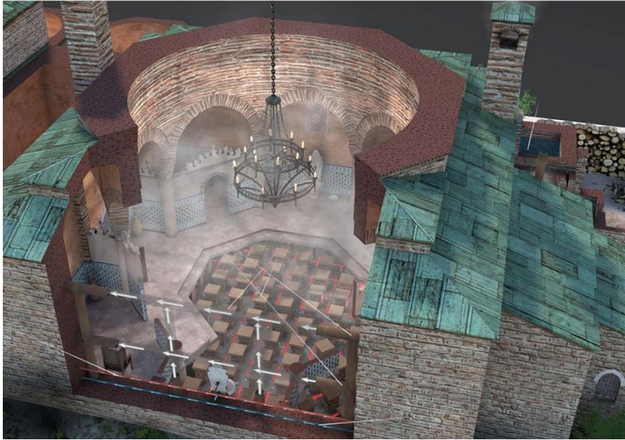
Figure 13 Thermal heating system- behind the walls (Mozaik Digital Education and Learning)
